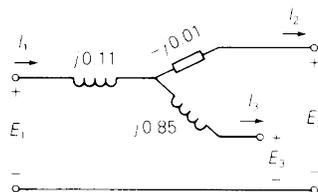
The per-unit equivalent circuit of this three-winding transformer is shown in Figure 3.21. Note that  $X_2$  is negative. This illustrates the fact that  $X_1$ ,  $X_2$ , and  $X_3$  are *not* leakage reactances, but instead are equivalent reactances derived from the leakage reactances. Leakage reactances are always positive.
