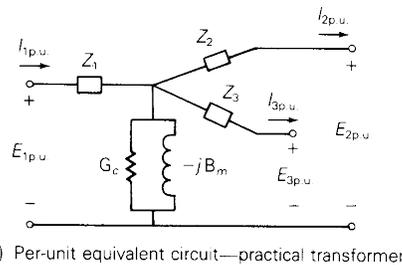
FIGURE 3.20 Single-phase three-winding transformer
